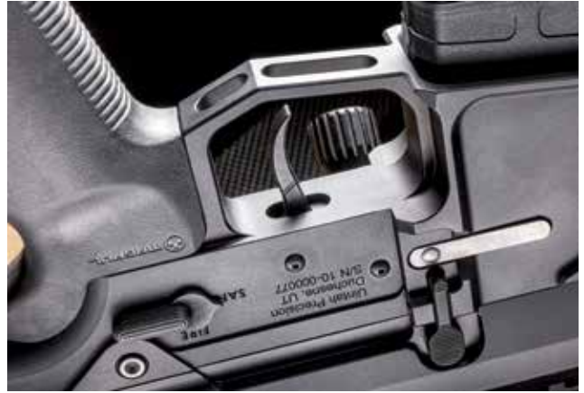
The single-stage trigger is Rise Armament's RA-535. It is a cassette-type trigger. The trigger fires after 3½ pounds of pressure. The lower is machined billet and the triggerguard is integral.
