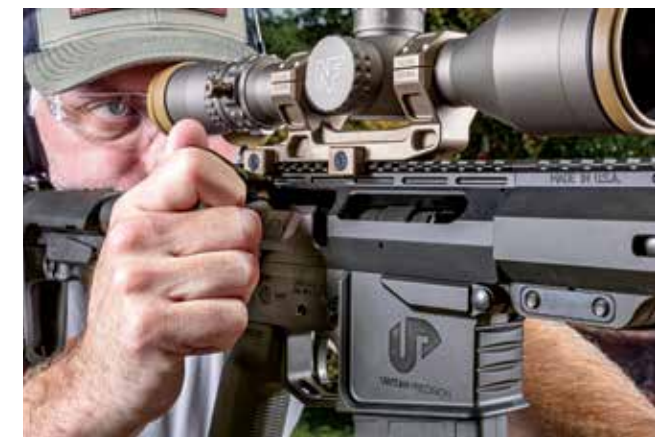
Due to the overall length of the bolt assembly, cycling the action feels abbreviated and quick. Unlike a gas-operated AR-pattern firearm with buffer assembly, this bolt only travels a few inches.
